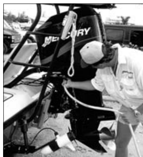
FISH, RINSE, REPEAT: Flushing the engine's cooling system with freshwater after use in saltwater is one of the most important things you can do to prolong engine life. Most engine manufacturers now offer built-in flushing ports that can be connected to traditional water hoses to make the process simple, although common "earmuff"-style portable flushers do a good job as well. Photo by Dan Armitage, for Lone Star Outdoor News.
