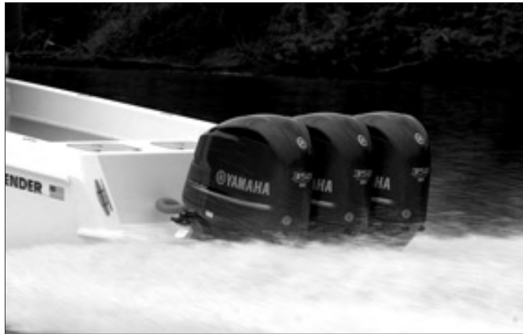
THREE OF A KIND: Yamaha's three F350 V-8 four-stroke motors pushed the test boat to 70 mph.
