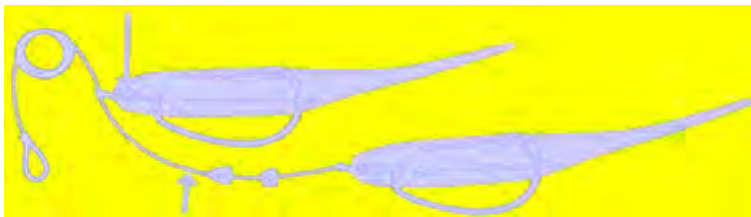
TRIED AND TRUE: SPI Lures' version of the speck rig incorporates swivels attached to the hooks and a clacker bead in between both lures. Graphic by SPI Lures.
